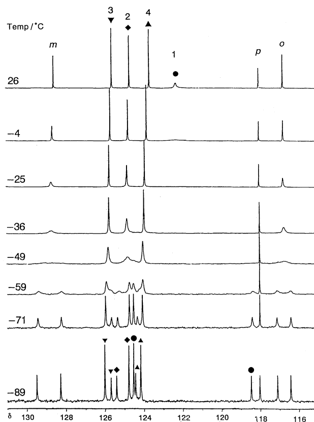
Figure 1. Temperature dependence of the tertiary aromatic carbon signals of compound 3 in CD 2 Cl 2 at 125 MHz.
